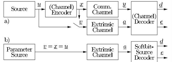
Fig. 2. a) Decoding model proposed in [2], [3]; b) modified model for SBSB.
