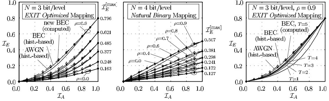
Fig. 3. EXIT-characteristics of SBSD, left/center: two examples for the dependency on  $\rho$  and the maximum values for  $\mathcal{I}_E^{\max}$ , right: dependency on  $T$ .
