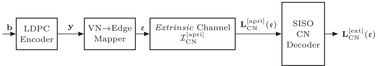
(b) Information theoretic transmission model for the EXIT chart analysis of the check node decoder.
