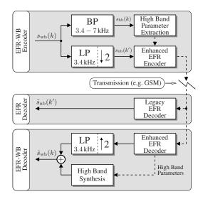
**Fig. 1.** Transmission system for backwards compatible wideband telephony using the GSM EFR narrowband codec [5].
