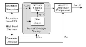
Fig. 2. Signal flow chart for high band synthesis.
