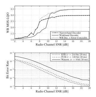
**Fig. 3.** Results of the GSM link-level simulations for the TU50 channel profile: Objective *wideband speech quality* (WB-PESQ) for narrow-/wideband decoders and *bit error rates* for all EFR bits, for the fixed codebook bits, and for the watermark bits.
