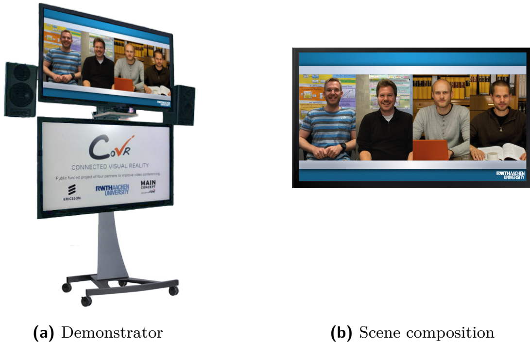
Figure 6.1: Real-time demonstrator setup and illustration of a scene composition of most active talkers in a video conference
