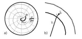
Fig. 3. a) Archimedes Spiral.  $r_n \ge 0$  solid,  $r_n < 0$  dashed. b) Decoding of a received symbol  $\underline{\tilde{x}}_a$  into  $\tilde{r_n}$
