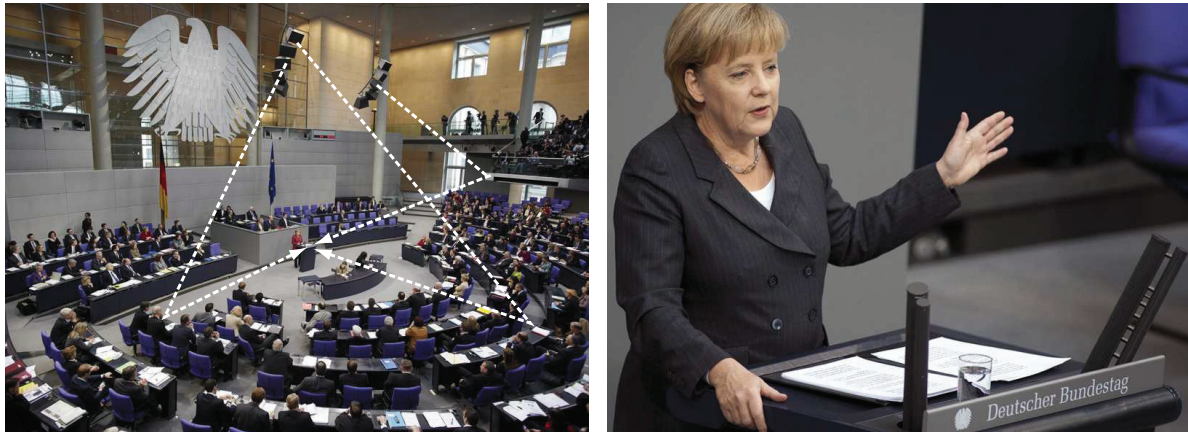
Figure 4.14: Pictures of the German Bundestag 2 . (left) Audience where the lines mark possible sound propagation paths from the loudspeaker system to the microphones at the lectern; (right) Speaker at lectern with two microphones.
