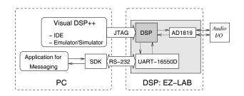
Fig. 2. Setup for real-time processing.
