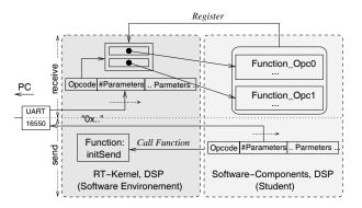
Fig. 4. Principles for sending and receiving runtime messages on the DSP side.
