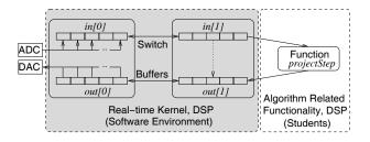
**Fig. 3.** Integration of the *projectStep* function into the software environment for signal processing.
