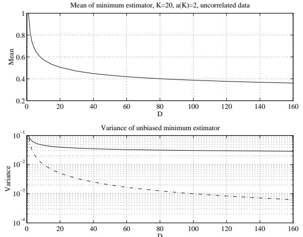
**Figure 3:** Mean (upper graph) and variance (lower graph, solid line) of minimum power estimate computed for uncorrelated data,  $\sigma^2(k) = 1$ ,  $K=20$ , and  $D=1-160$  (Dashed line gives minimum variance achieved by non recursive smoothing over  $K \cdot D$  segments).
