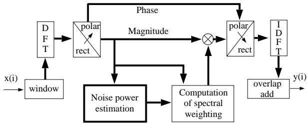
Figure 2: Block diagram of spectral processing
