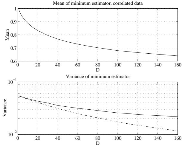
**Figure 4:** Mean (upper graph) and variance (lower graph, solid line) of minimum power estimate computed for correlated data with  $\sigma^2(k) = 1$ ,  $\alpha = 0.95$ , and  $D=1\text{--}160$  (Dashed line gives variance for non recursive smoothing of  $D$  short time power estimates).
