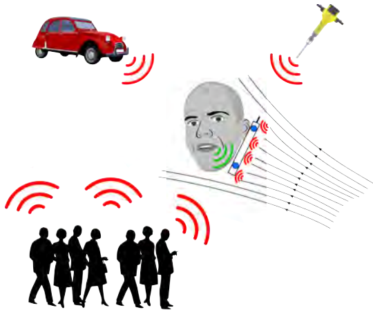
Figure 2.1: Wind and background noise scenario for a mobile phone with two microphones.
