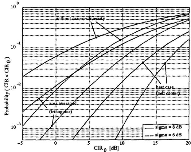
Figure 6. Impact of different  $\sigma$ ; maximal ratio combining, uncorrelated paths
