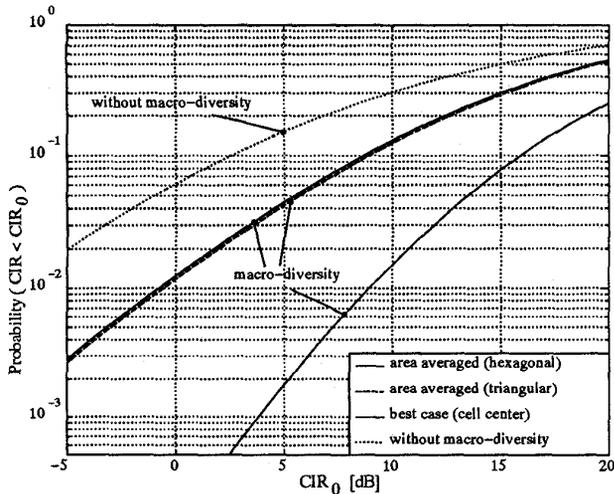
Figure 5. Outage probabilities for systems with and without macro-diversity; maximal ratio combining, standard deviation of shadowing  $\sigma = 8$  dB, uncorrelated paths
