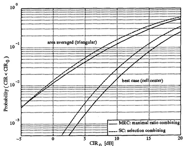
Figure 7. Comparison of maximal ratio and selection combining;  $\sigma = 8$  dB, uncorrelated paths
