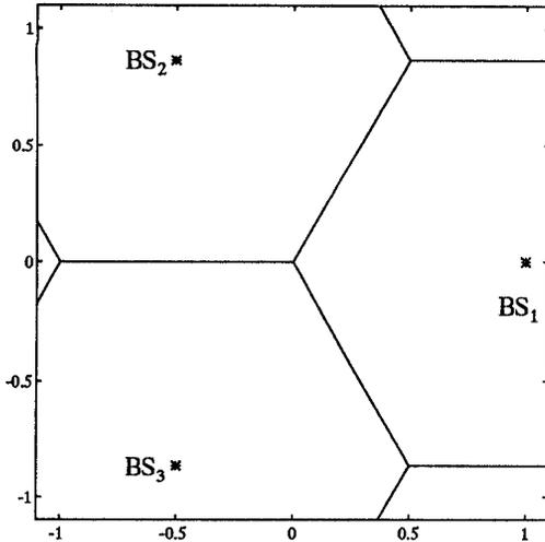
Figure 3. Considered cell area for conventional hexagonal cells
