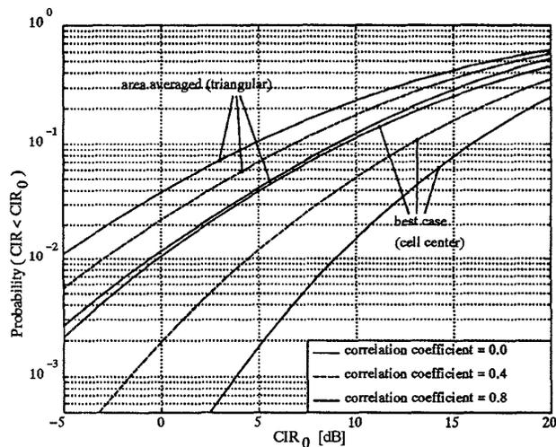
Figure 8. Comparison for different correlation coefficients; maximal ratio combining,  $\sigma = 8$  dB
