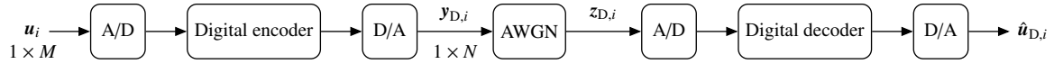
Figure 2: Purely digital transmission system with a source vector captured by microphone i .
